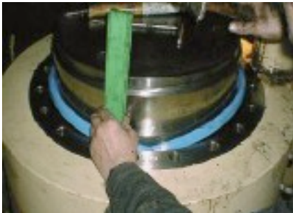
Fitting a split seal to a multi-opening press
