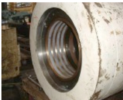
Repaired bush of single-opening PB press
