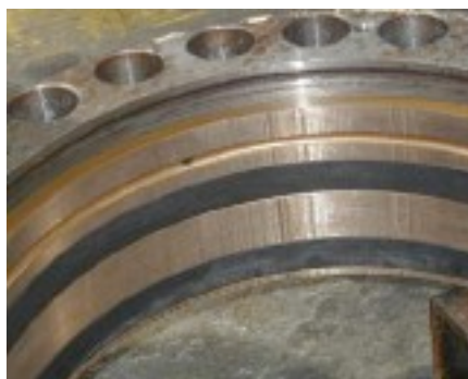
Repaired bottom bush of laminating press
