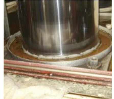
Left: Worn bushing from a multi-daylight press
